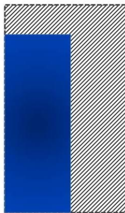
Figure 2: Blue shaded area shows the reduced footprint of the ZW1500-RMS when compared to a typical pressurized UF rack.
